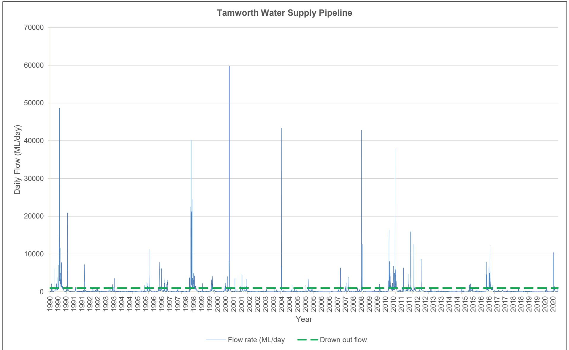
Figure 36. Fish passage availability at Tamworth Water Supply over a 30 year period. Green line indicates approximate flow volume at which fish passage is possible
