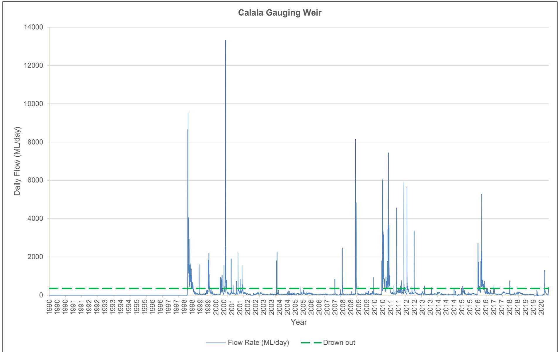
Figure 35. Fish passage availability at Calala Gauging Weir over a 30 year period. Green line indicates approximate flow volume at which fish passage is possible
