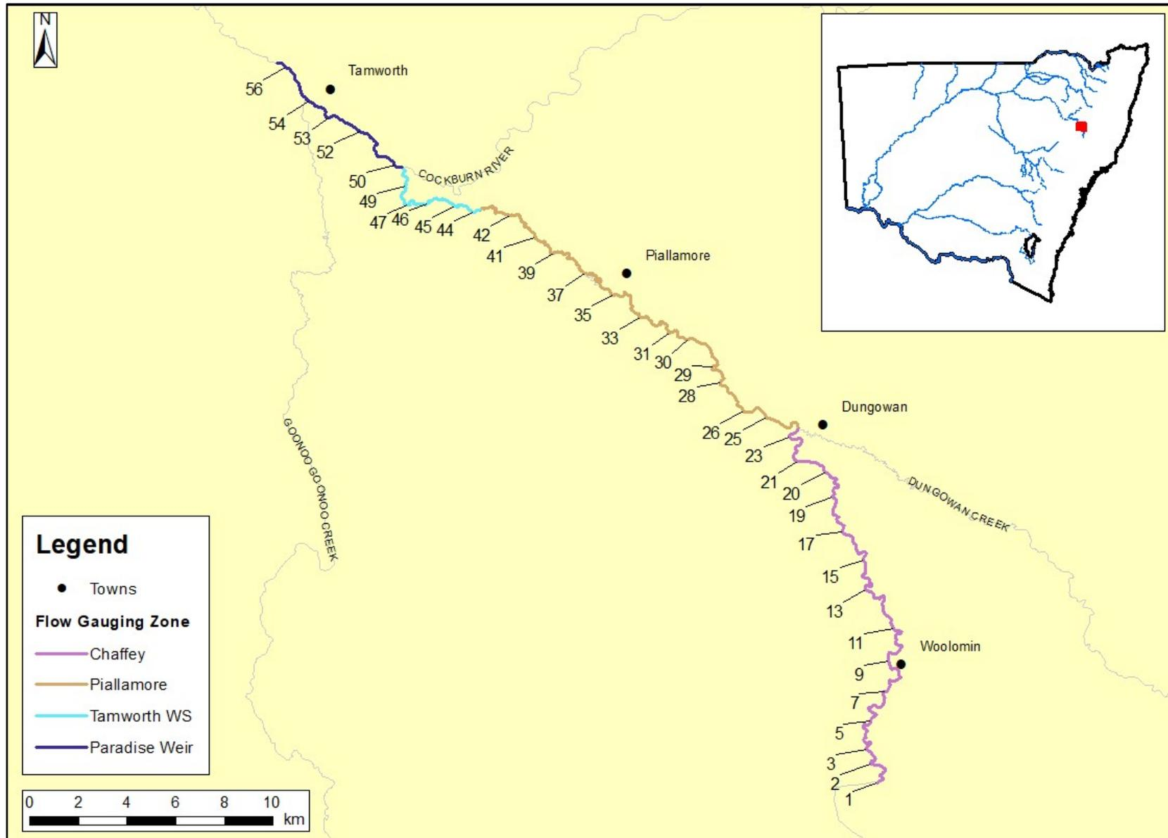
Figure 26: Flow Gauging Zone boundaries used during the project to assess flow relationships for habitat features during the project
