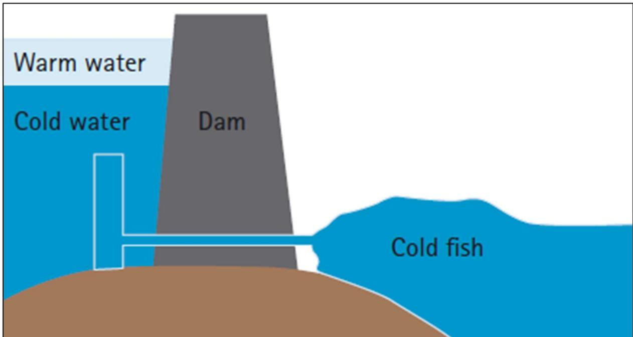
Figure 41. Cold water pollution occurs through drawing of water from the bottom of large storages (NSW DPI, 2005).
