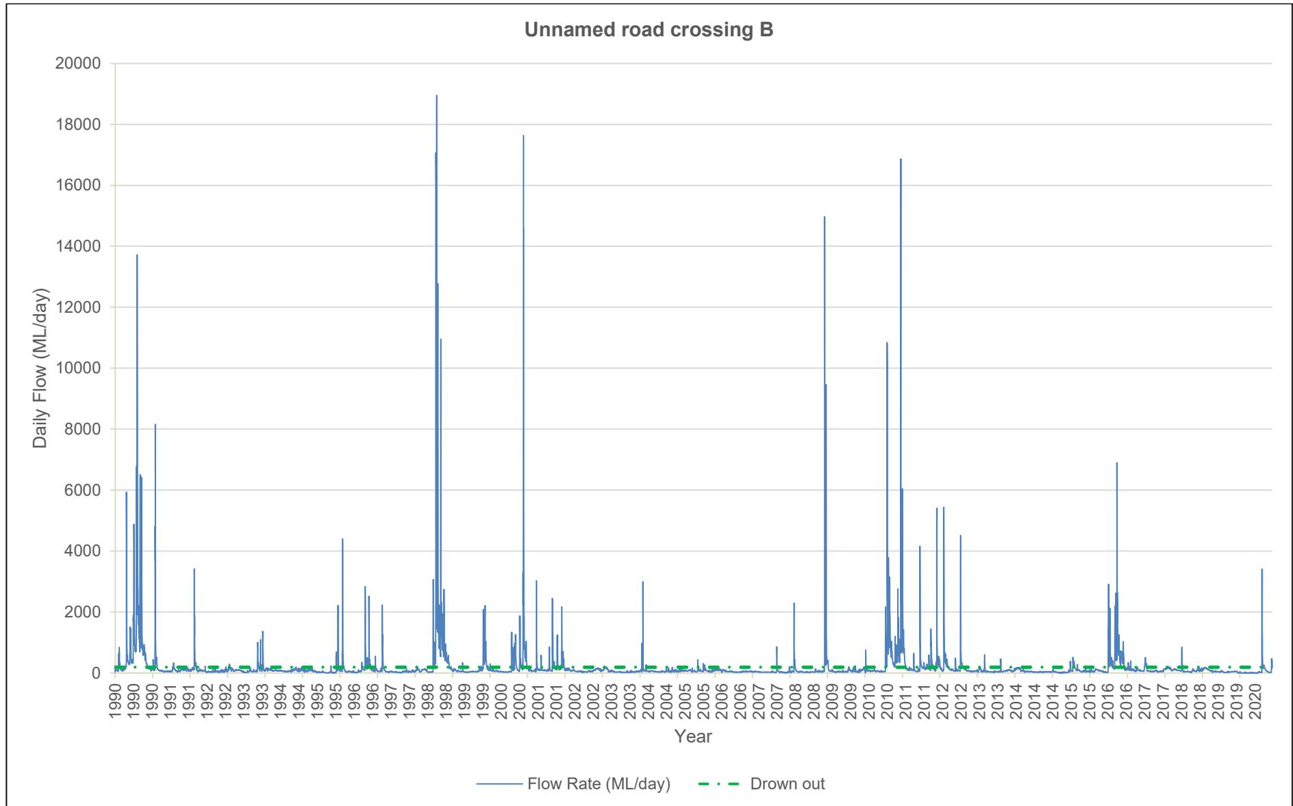
Figure 34. Fish passage availability at Unnamed road crossing B over a 30 year period. Green line indicates approximate flow volume at which fish passage is possible. \*One flow value (30,000 ML/day) in November 2000 was removed to allow finer flow – axis resolution
