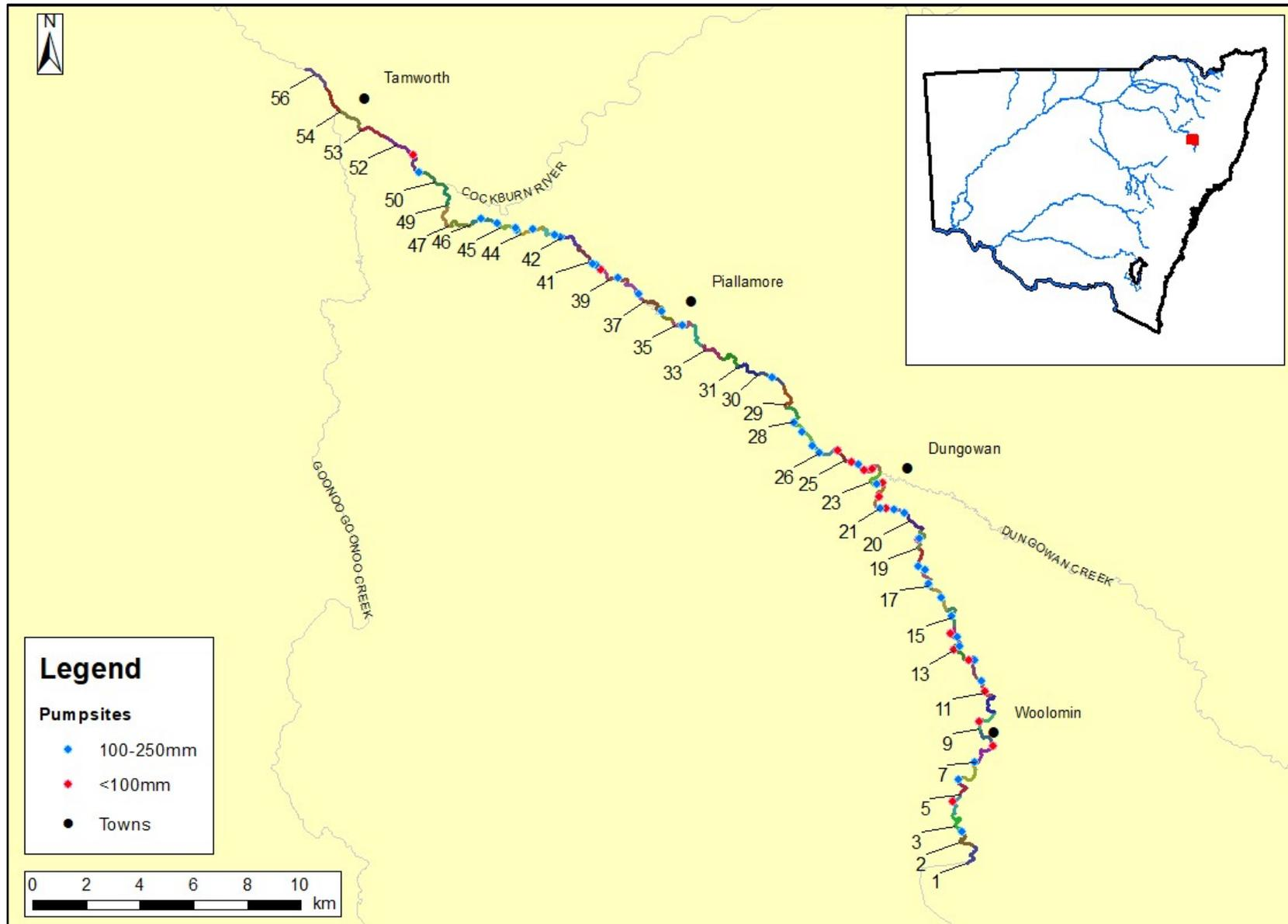
Figure 38. Pumpsite distribution and diameter in the project area
