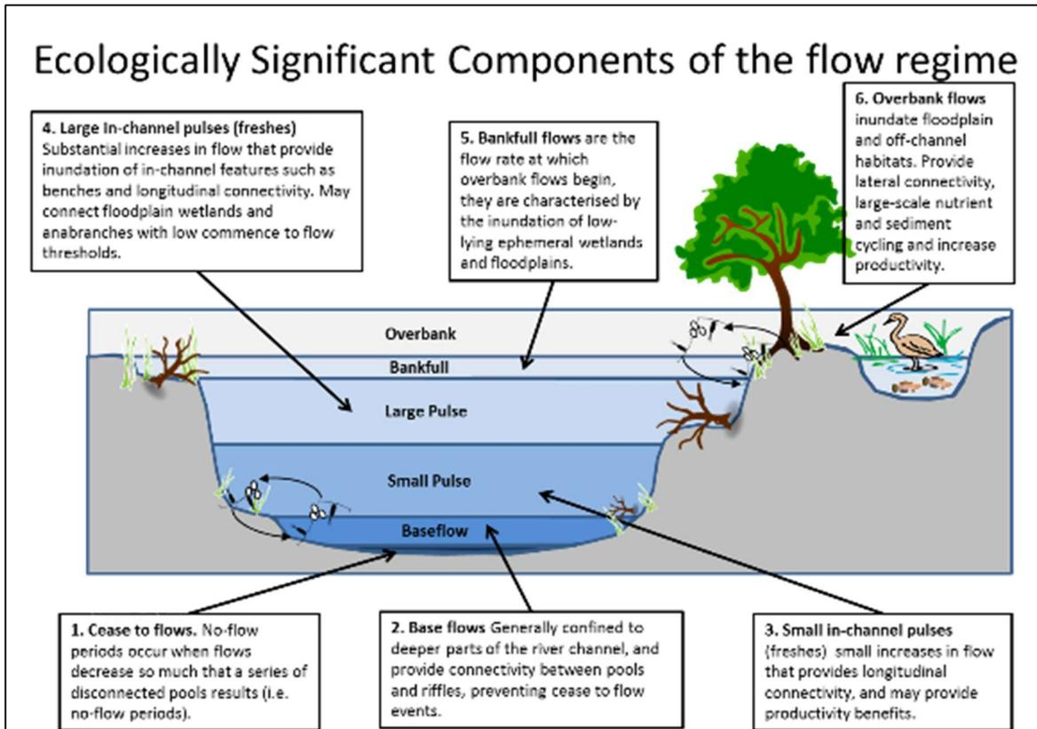
Figure 25. Components of the within-channel flow regime (adapted from Ellis et al. 2016)
